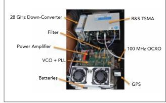
justed to the sup-  $\triangle$  Fig. 5 R&S 5GTF coverage measurement system.
