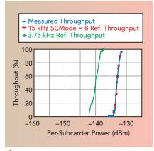
Fig. 7 Simulated throughput for the in-band NB-IoT mode.
