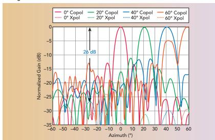
Fig. 4 256 element transmit cuts at 28 GHz over full scan showing greater than 26 dB isolation.
