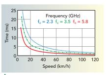
Fig. 2 Coherence time vs. speed for three carrier frequencies below 6 GHz.
