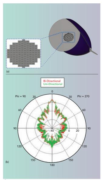
▲ Fig. 1 Antenna array inside a radome (a) and simulated patterns (b).
