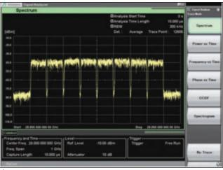
▲ Fig. 2 The MS2850A can measure up to eight 100 MHz bandwidth carriers, here centered at 29 GHz.
