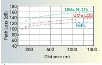
Fig. 3 28 GHz path loss vs. cell separation, comparing FSPL with LOS and NLOS for an urban macro deployment, using the ABG channel model.
