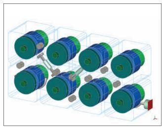
▲ Fig. 2 Cross-coupled dielectric resonator filter tuned with the Filter Designer 3D optimizer.
