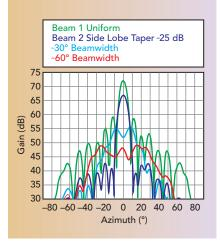
Fig. 2 Beam gain for four preselectable states of the active array.
