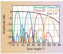
Fig. 3 Scan roll-off factor from 0 to 60 degrees.
