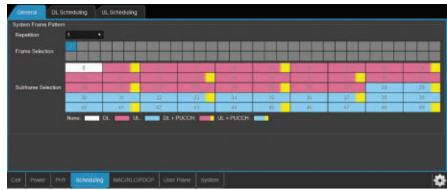
Fig. 3 GUI for configuring subframe patterns.
