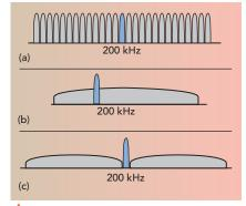
Fig. 2 Deployment modes for NB-IoT: standalone GSM (a), in-band LTE (b) and guard-band LTE (c).
