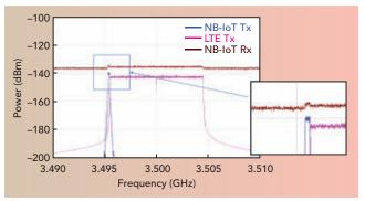
Fig. 8 NB-IoT and LTE spectra for the guard-band mode.
