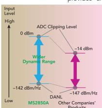
▲ Fig. 1 The ADC clipping level of 0 dBm enables the MS2850A to have a measurement dynamic range greater than 140 dB at 1 GHz.
