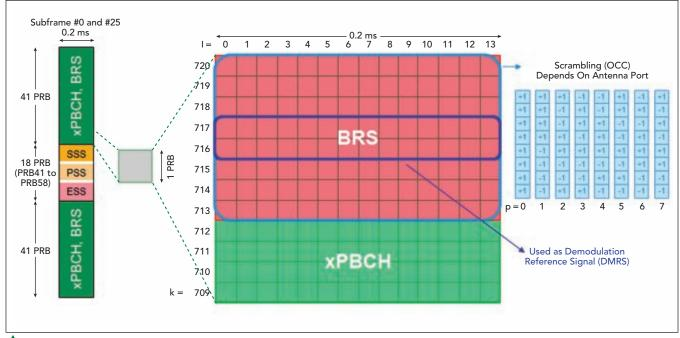
Fig. 4 5GTF synchronization and beamforming reference signals.
