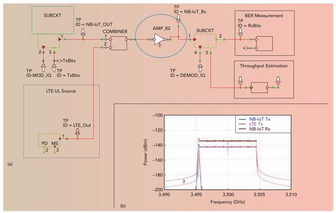
Fig. 9 Test bench with power amplifier (a) and guard-band mode spectra (b).
