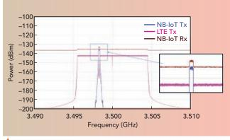
Fig. 5 NB-IoT and LTE spectra for the in-band mode.
