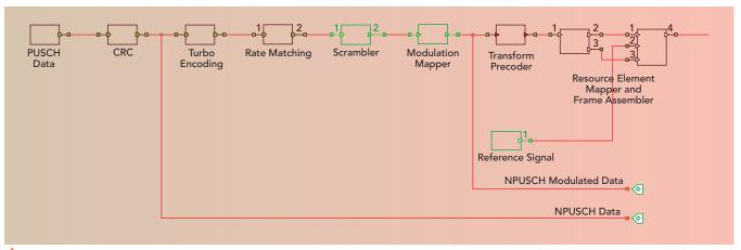
Fig. 4 NPUSCH encoder simulated in VSS.
