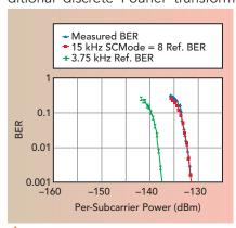
Fig. 6 Simulated BER for the NB-IoT signal passed through AWGN channel model.
