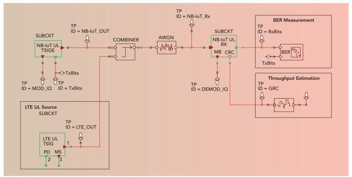
Fig. 3 Test bench for the NB-IoT in-band uplink mode.
